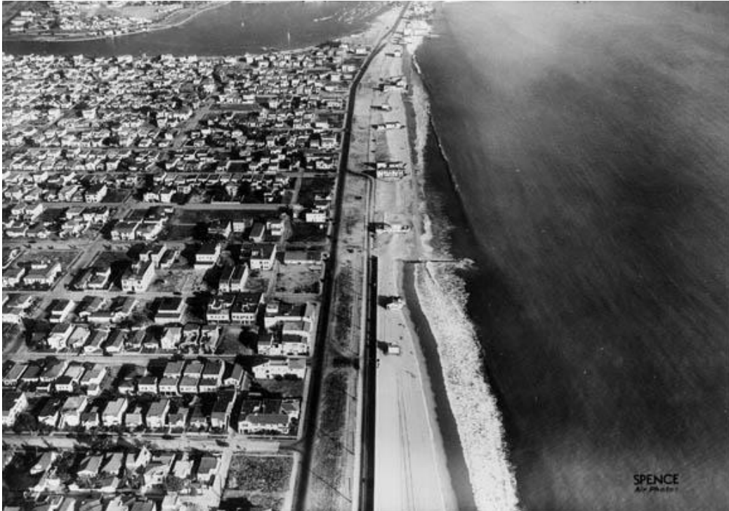
Belmont Shore, 1945. Aerial photograph shows Ocean Boulevard with old Pacific Electric right of way in the center and two separated one-way roadways.
